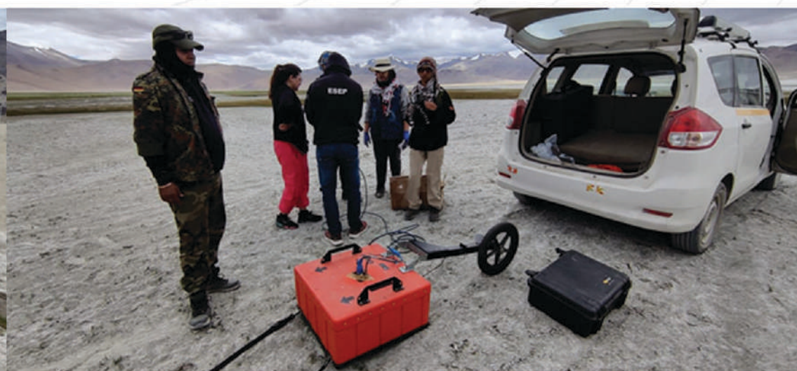
Sampling and measurement of site parameters and Ground Penetrating Radar (GPR) to explore the subsurface of the Tso Kar basin.
